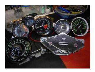
British speedometers: I can correct for ratio changes in the instrument too some degree with worm drive and gear combinations both odo and speed pointer.
